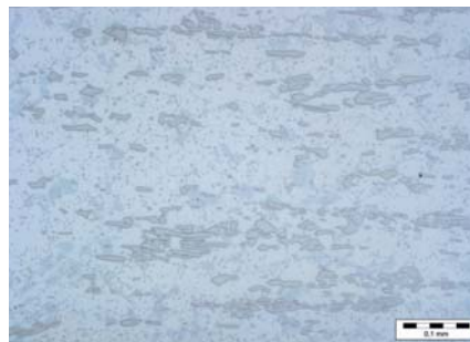
Fig. 6: Cold work tool steel after initial hot forming, slightly contrasted by a short final oxide polish, showing large primary carbides in a ferritic-pearlitic matrix 200x
