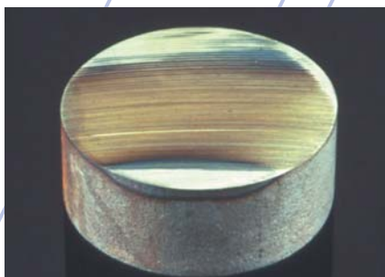
Fig. 1: Thermal damage due to faulty cutting conditions
