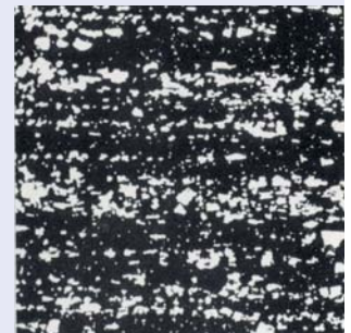
Fig.11: Carbide distribution in conventionally produced steel
