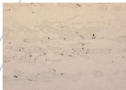
Fig. 2: Fractured primary carbides
