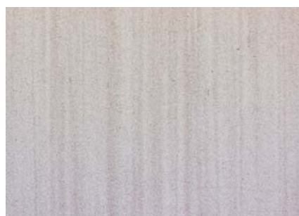
Fig. 8: Hot work tool steel showing segregations 100x
