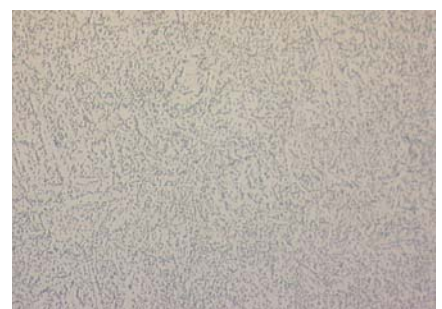
Fig. 5: Hot work tool steel etched with Picral and Nital, globular pearlite
