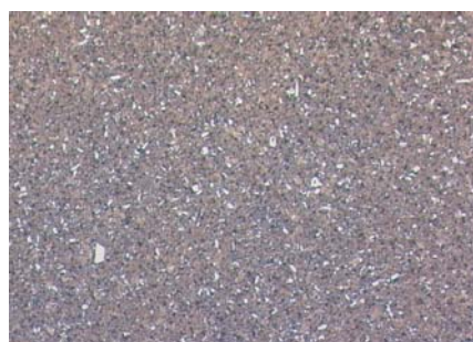
Fig. 4: Cold work tool steel etched with 10% Nital, primary carbides stand out white
