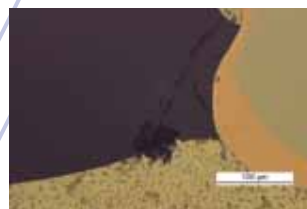
Fig. 4: Crack and fracture damage in glass diode caused by coarse grinding paper
