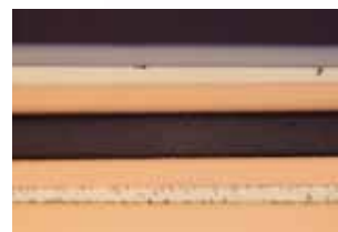
Fig. 5: Relief from polishing due to different hardness of materials
