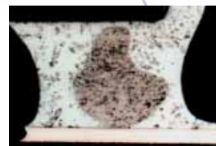
Fig. 6: Diamond particles in solder
