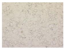
Fig. 8: Austenite with carbides and some 200x titanium carbon nitrides
