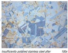
Insufficiently polished stainless steel after colour etching (Beraha II), showing deformation
