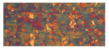
Fig.2: Austenitic steel, colour etched (Beraha II).
