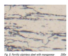
Fig. 5: Ferritic stainless steel with manganese sulfides and strings of small carbides, etched electrolytically with 10% oxalic acid
