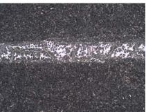
Fig. 6: Tempered martensitic stainless steel with delta ferrite, etched with picric acid
