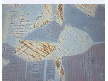
Fig. 3: Austenitic steel insufficiently polished showing deformation after etching (Beraha II)
