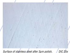
Surface of stainless steel after 3µm polish, showing deformation from grinding
