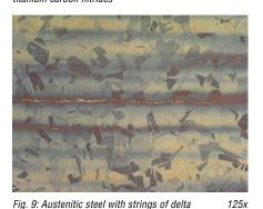
Fig. 9: Austenitic steel with strings of delta ferrite, showing microsegregations.
