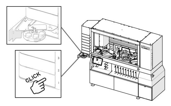
4. The machine automatically detects the specimen holder.
