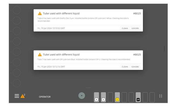
You can also initiate cleaning yourself when you find this necessary, or if the machine is not going to be used for a period of time. You can select functions to clean one or all tubes from the bottles to the dosing nozzles, either from the main menu or during the process.
