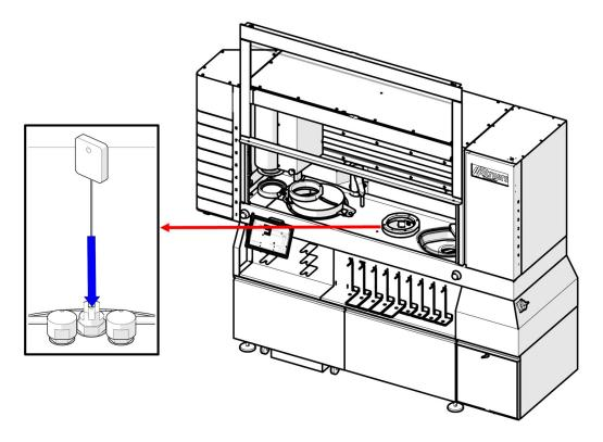
• Use the nozzle cleaner to clean the nozzles in the high pressure cleaning station.
