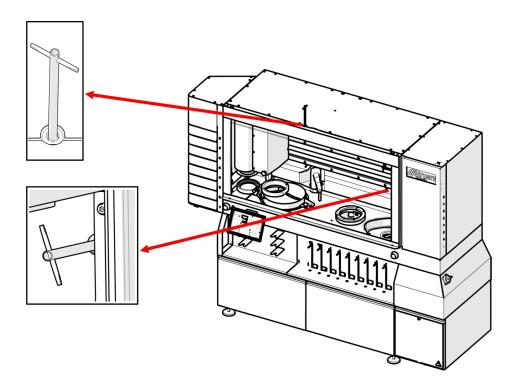
3. Turn the key clockwise to open the main safety cover and the MD elevator.
