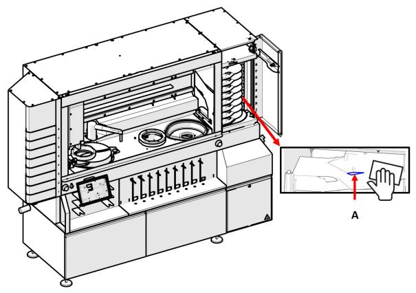
• Clean the mirrors (A) inside the 8 drawers in the MD surface elevator with a damp cloth.
