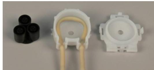
5. Remove the Novoprene tube.
