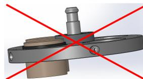
1. Place at least three specimens symmetrically around the center of the specimen holder so that you achieve an even and balanced rotation.
