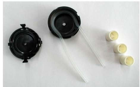
5. Remove the Novoprene tube.
