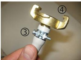
Place the screw clip ③ onto the hose.
