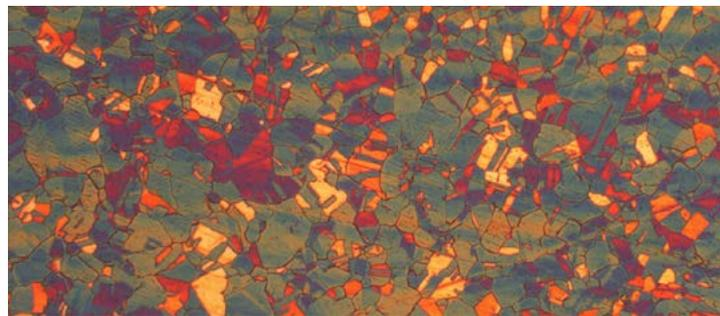
Fig.2: Austenitic steel, colour etched (Beraha II).
