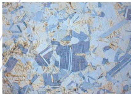
*Insufficiently polished stainless steel after colour etching (Beraha II), showing deformation 100x*
