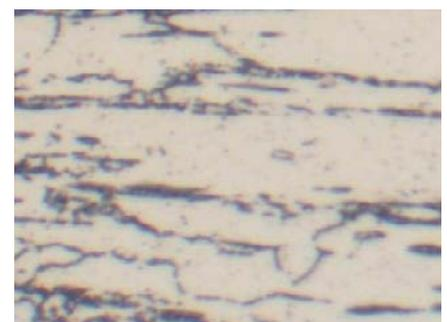
Fig. 5: Ferritic stainless steel with manganese sulfides and strings of small carbides, etched electrolytically with 10% oxalic acid 200x
