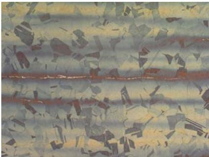
Fig. 9: Austenitic steel with strings of delta ferrite, showing microsegregations. Blue areas: depletion of alloying elements. 125x
