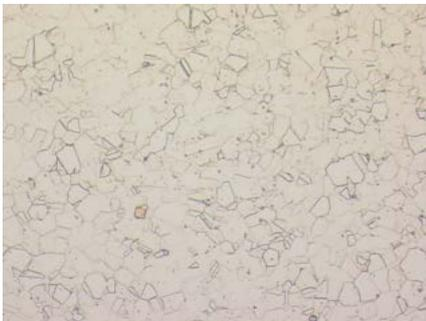
Fig. 8: Austenite with carbides and some titanium carbon nitrides 200x
