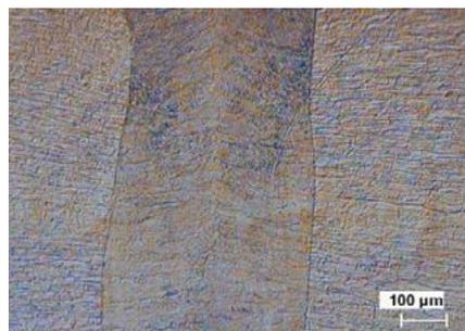
Fig. 4: Stainless steel weld, polished and etched electrolytically, DIC
