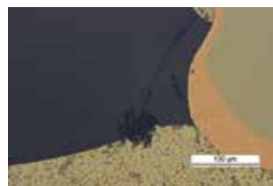
Fig. 4: Crack and fracture damage in glass diode caused by coarse grinding SiC Foil/Paper
