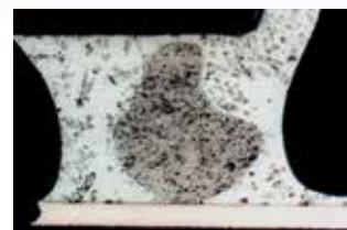
Fig. 6: Diamond particles in solder
