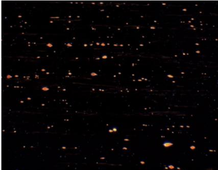
Fig. 5: Copper with red copper oxides,
