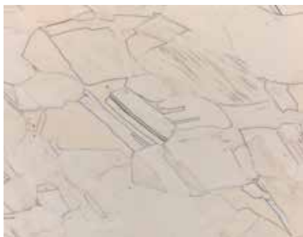
Fig. 6: Oxygen free copper, etched with ammonium peroxydisulfat, 100x.
