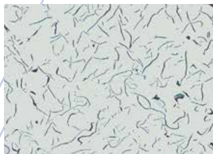
Fig. 2: Same as Fig.1, showing correct polish
