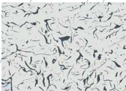
Fig. 1: Grey iron with flake graphite, insufficient polish
