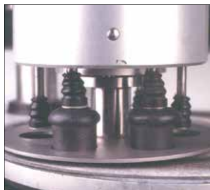
Fig.13: Sample holder for semi-automatic polishing of quality control samples in cast line
