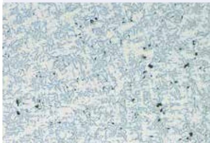
Fig. 3: Grey iron with fine flake graphite, unetched 100x
