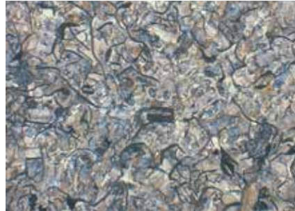
Fig. 4: Grey iron with flake graphite in pearlitic matrix 200x
