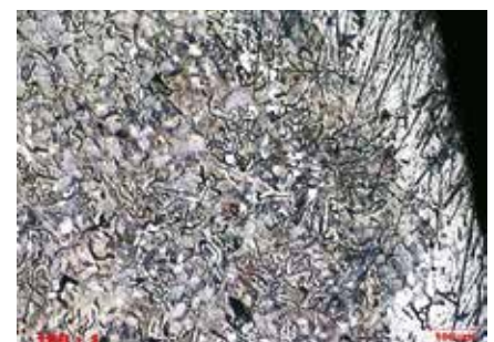
Fig.16: Grey iron prepared with fine grinding on silicon carbide Foil/Paper, still shows scratches
