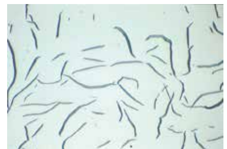
Fig.14: Well polished graphite flakes 500x
