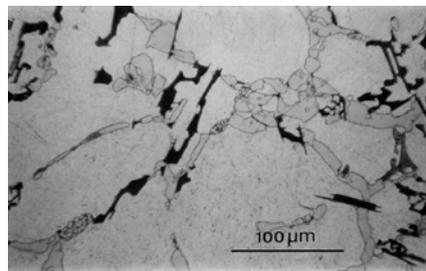
Fig. 16: Same as Fig. 15 but etched for 30 sec with 1g molybdic acid in 200 ml water + 6g ammonium chloride. The silicon is dark blue and is distinguishable from the greyish CuAl<sub>2</sub>.
