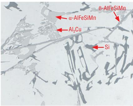
Fig. 6: AlSi6Cu4 cast, the various phases can be identified by their typical colour.
