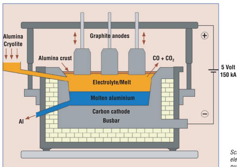
Schematic drawing of the electrolysis producing pure aluminium.
