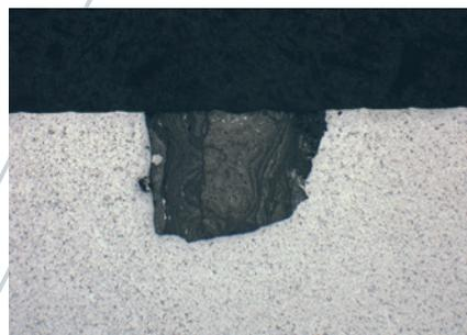
Fig. 2: Oxide in the surface of an aluminium pressure die casting, 50x.
