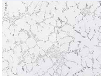
Fig. 10: Structure as in Fig. 9, but fine polished with OP-U suspension. The matrix is well polished and the eutectic has more contrast, 200x.
