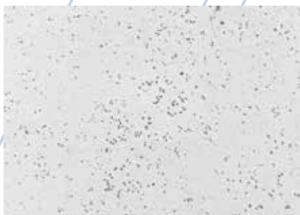
Fig. 1: Embedded diamond particles in pure aluminium after polishing with 3 µm, 200x.
