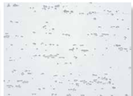
Fig. 5: As Fig. 4, hot rolled, unetched, 200x.
