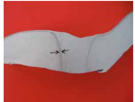
Fig.13: Pressed part, macro etching, primary and heterogeneous precipitates are revealed that have a negative effect on the surface of the final product.
