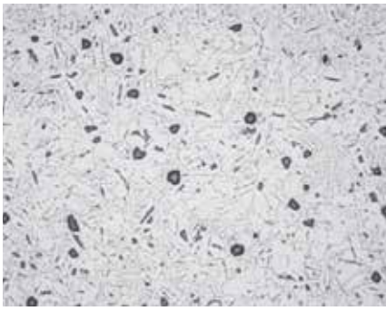
Fig.11: Aluminium-silicon cast polished too long with OP-S suspension, silicon precipitates stand in relief, 100x.
