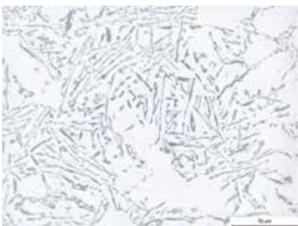
Fig. 7: Aluminium-silicon cast, unrefined, 500x.
