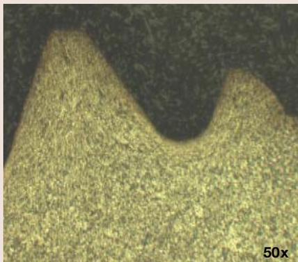
Thread of bolt, alloyed steel tempered
