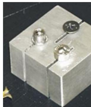
Fig. 3: Special holder for cutting screws
