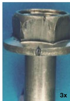
Fig. 7a: Split in head of carbon steel bolt caused by a seam.
