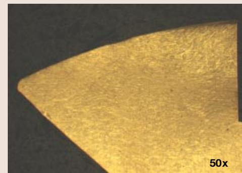
Head of brass screw with flow lines from cold forming. Echant: Iron (III) chloride
