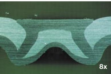
*Riveted joint, steel rivet in aluminum*
