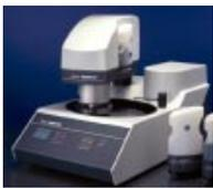
The coarse grinding to the middle of the screws was carried out on the Struers automatic grinding machine Abraplan, the subsequent automatic fine grinding and polishing on Struers TegraPol.
