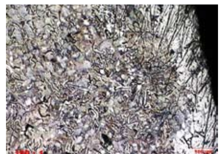
Fig. 16: Grey iron prepared with fine grinding on silicon carbide paper, still shows scratches
