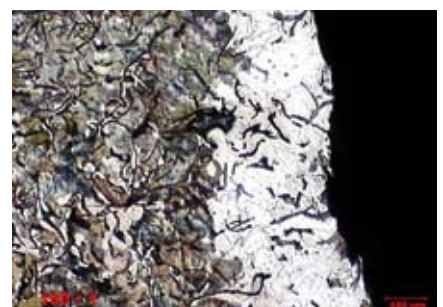
Fig. 17: Same as Fig.16, prepared with fine grinding with diamond on MD-Largo, showing good edge retention
