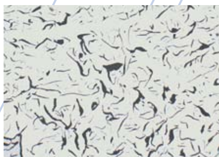
Fig. 1: Grey iron with flake graphite, insufficient polish
