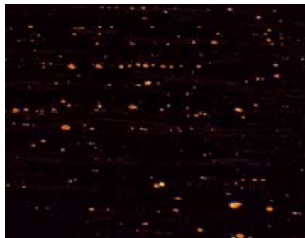
Fig. 5: Copper with red copper oxides, dark field, 500x.
